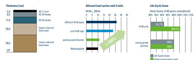
Our OMV Starfalt<sup>®</sup> PmB is not only used for motorway or express way construction. This excellent binder proofs its quality already many times for the construction of airfields like taxiways and runways. Started in 1990 with the reconstruction of the runway of the military airfield in Zeltweg it continues the years after. Since 2010 our PmB has been used during rehabilitation projects for a significant number of airports:
